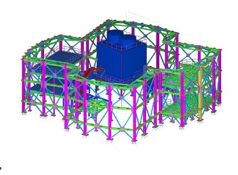
Using the 3D modelling software, Tekla®, we are able to produce models of any structure to be fabricated.
